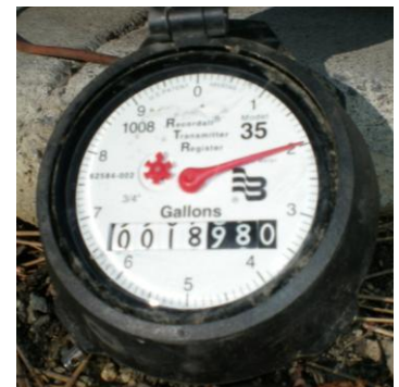
Water Meter Register
